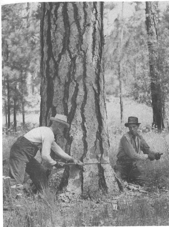
Figure 14.1 Felling a large diameter ponderosa pine using a crosscut saw Colville Indian Reservation, Washington. Original caption, "Felling crew at work on the Katar unit, ca. 7/1942." Source: Harold Weaver/ U.S. National Archives and Records Administration (NARA)/Wikimedia Commons/Public Domain.
